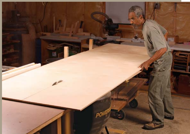
Push. The cart supports the back end of the plywood, freeing you up to feed the material and apply pressure against the fence.
