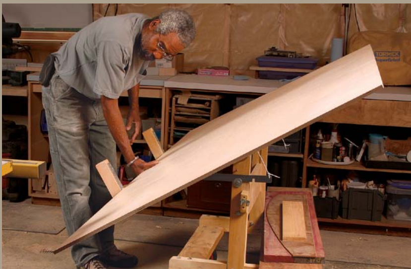
Pivot. Tip the support frame that holds the sheet goods into the horizontal position, where it locks automatically. Then move the cart into position and apply the brake.
