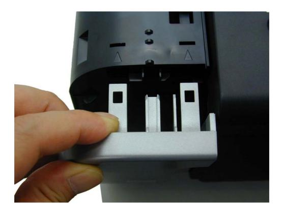
(IV) Release the 2 hooks on the rear side of the printer (indicated by the blue circles).
