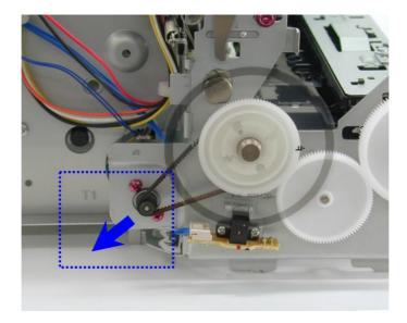
Note: The red screws securing the paper feed motor may be loosened only at replacement of the paper feed motor unit. DO NOT loosen them in other cases.
