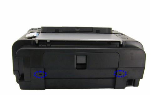
(V) Release the hook on the left side of the printer, then while inserting the flat-blade screwdriver in the slots on the left and right sides of the printer front, release the hooks to remove the main case from the bottom case.
