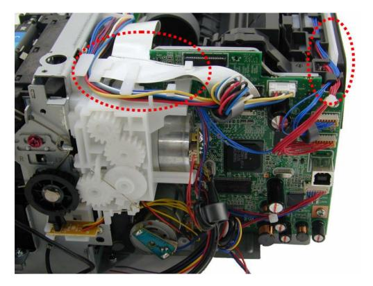
(II) Paper feed motor side wiring
