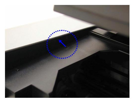
(II) Remove the screws (at 2 locations) and the flexible cable (at 1 location).
