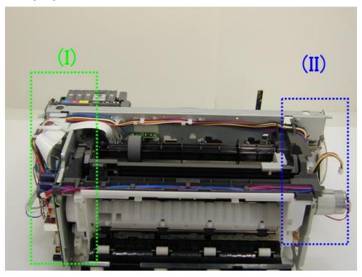
(I) Front cover right unit and logic board ass'y wiring
