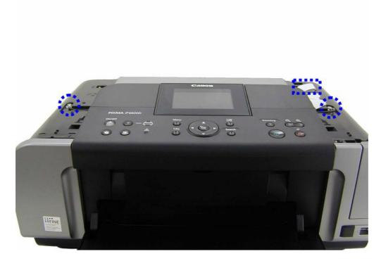
(III) Release the hooks and remove the front left cover as shown below.
