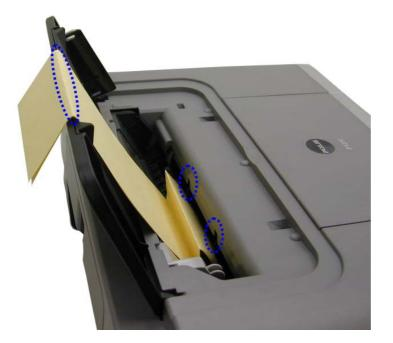
4) Press and hold the Stop/Reset button until the Power LED blinks 3 times, then release the button to perform the paper feed roller cleaning. See "Standalone printer operation," for details.
