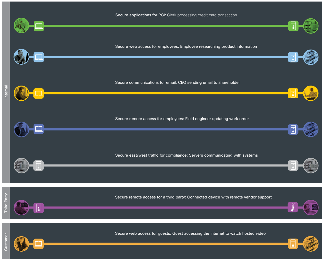
Figure 4 Data center business flows map to functional controls based on the types of risk they present.
