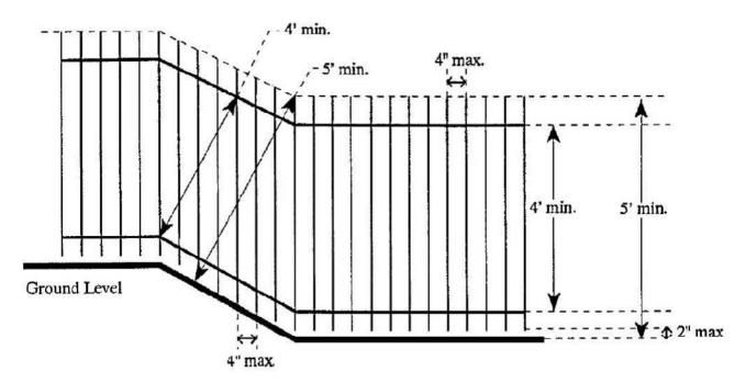
Figure 318-4 Perpendicular fencing dimensions on sloping ground.
