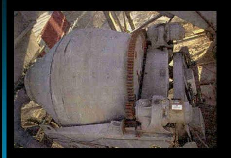
The work of the torque (or moment) developed by the driving gears on the two motors on the concrete mixer is transformed into the rotational kinetic energy of the mixing drum.
