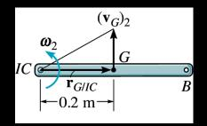
At position 2, point A is the instantaneous center of rotation. Hence,  $v_{G2} = r \omega = 0.2 \omega_2$ .
