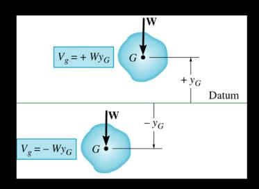
The gravitational potential energy of a body is found by the equation
