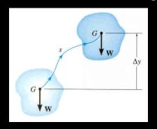
Work of a weight: As before, the work can be expressed as  $U_w = -W\Delta y$ . Remember, if the force and movement are in the same direction, the work is positive.
