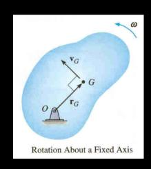
2. Pure Rotation: When a rigid body is rotating about a fixed axis passing through point O, the body has both translational and rotational kinetic energy. Thus,
