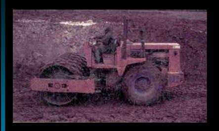
Are the kinetic energies of the frame and the roller related to each other? How? The work done by the soil compactor's engine is transformed into the translational kinetic energy of the frame and the translational and rotational kinetic energy of its roller and wheels (excluding the additional kinetic energy developed by the moving parts of the engine and drive train).
