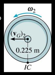
$$T_2 = 0.5 \text{m } (v_{G2})^2 + 0.5 I_G (\omega_2)^2$$
