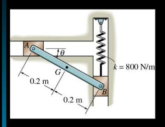
Given: The rod AB has a mass of 10 kg. Piston B is attached to a spring of constant k = 800 N/m. The spring is un-stretched when  $\theta = 0^{\circ}$ . Neglect the mass of the pistons.
