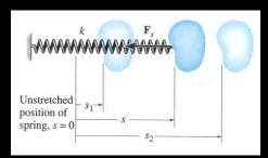
Work of a spring force: For a linear spring, the work is
