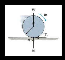
Normal forces and friction forces acting on bodies as they roll without slipping over a rough surface also do no work since there is no instantaneous displacement of the point in contact with ground (it is an instant center, IC).
