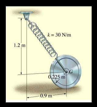
Given: The weight of the disk is 150 N and its k<sub>G</sub> equals 0.18 m. The spring has a stiffness of 30 N/m and an unstretched length of 0.3 m.
