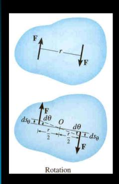
When a body subjected to a couple experiences general plane motion, the two couple forces do work only when the body undergoes rotation.
