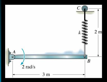
Given: A 50 N bar is rotating downward at 2 rad/s. The spring has an unstretched length of 2 m and a spring constant of 12 N/m.
