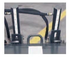
The **depth of the skis** is indicated by a depth gauge visible from the operator seat.
