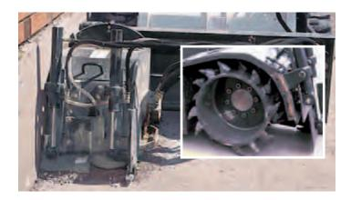
The **right ski and end plate** are removable to allow flush milling against curbs or walls (14", 16", 18" and 24" drum). Side cutting bits decrease drum binding and provide a vertical edge for improving the joint bond.
