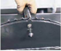
The **planer housing** oscillates  $\pm 15^{\circ}$  for cutting at an angle or matching uneven surfaces. An indicator is provided with markings locating each  $\pm 5^{\circ}$  of oscillation. If desired, it may be put in a locked position.
