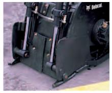
**Dual cylinders**, independently adjustable, provide depth control for each ski.\*\*
