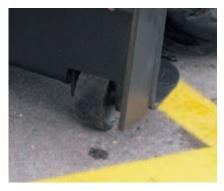
**Steel wheels** mounted on the rear frame help support the planer when starting a cut and while planing.
