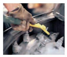
The **top access service panel** is of sufficient size to replace the cutting bits without raising the planer from the surface or removing the drum.
