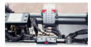
Individual ski depth gauge and oscillation gauge are easily visible from the operator seat.
