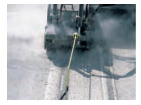
Optional guide rod available for 14", 16", 18" and 24" Bobcat planers; helps the operator maintain a straight cut.
