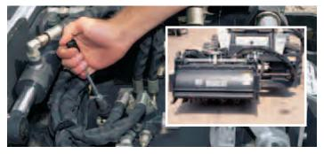
Use the diverter valve control to switch between hydraulic side-shift and hydraulic oscillation.
