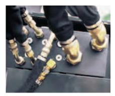
The high-flow planer attachment utilizes a **priority valve** to divert oil to depth functions without causing momentary loss of power to the planer drum; this allows the operator to make adjustments on the go.\*\*
