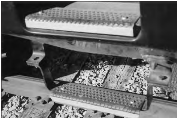
TRACTION TREAD™ was used to make non-slip, gripping stair treads for this railroad locomotive.
