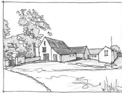
Informal arrangement of steading/courtyard, Lean-to's, informal openings, shelter, mature tree's, prominent gable with large openings, clipped eaves.
