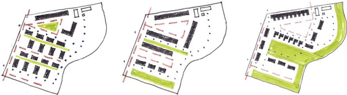
Examples of density & road layout analysis; to achieve the most resource efficient form of development
