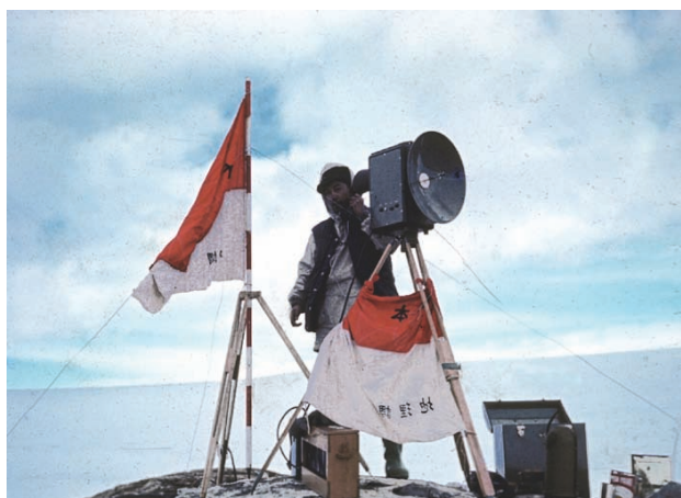
Photo 1 Observation by microwave distance meter, Tellurometer (JARE-4)
