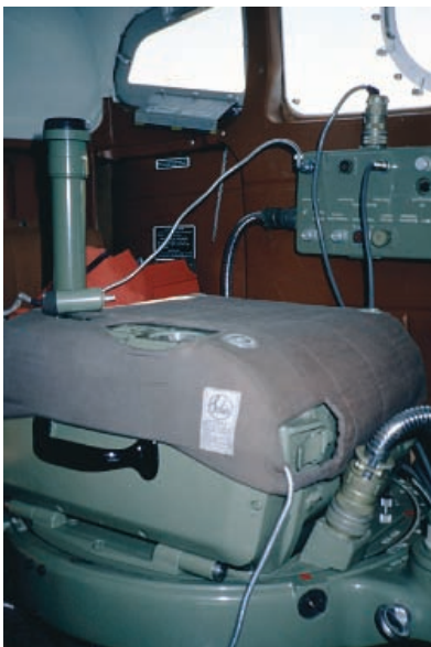
Photo 5 Aerial camera, RC-9, installed in a Cessna
