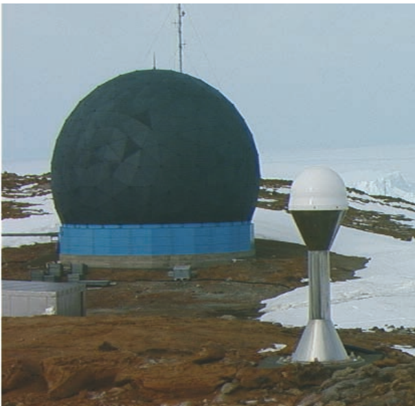
Photo 12 Multipurpose antenna at Syowa Station (In the redome at the back, the GPS continuous observation station is at the forefront.)
