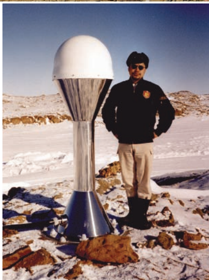
Photo 10 Pillar antenna of continuous GPS observation station and other observation facilities of the surrounding area
