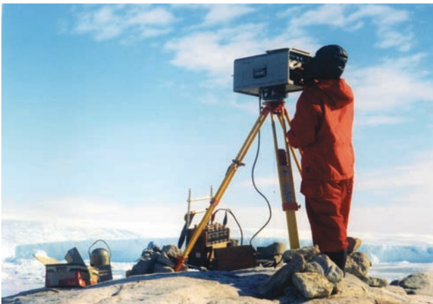
Photo 4 Observation by electro-optical distance meter, Geodimeter 8 (JARE-14)
