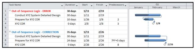
Figure 9.1.1-4 Impact of Out-of-Sequence Logic
