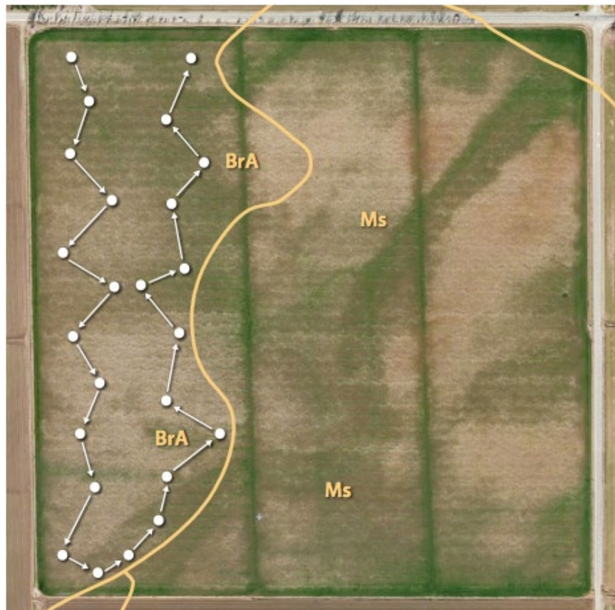
Figure 5-4 Soil sampling plan to obtain a representative sample from a field or management area. The sampling points are shown on a Google map using the SoilWeb application (available at casoilresource.lawr.ucdavis.edu/soilweb/ ).
