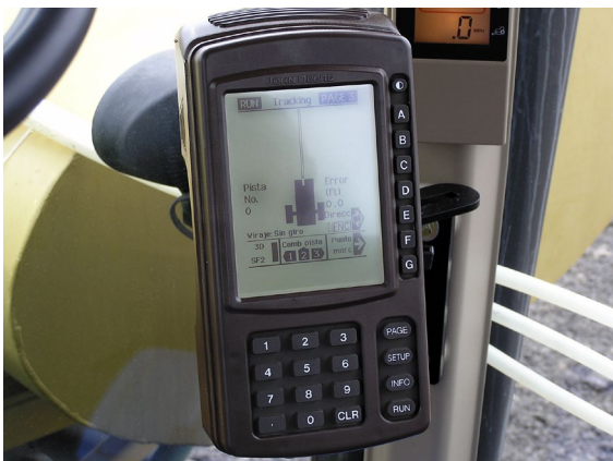
Figure 4-6 Use a tractor-mounted GPS to help you apply pesticides evenly, without overlaps or gaps.
