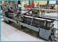
**Geared Head Toolroom Engine Lathe**
