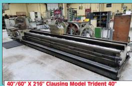
40"/60" X 216" Clausing Model Trident 40 Geared Head Gap Bed Toolroom Engine Lathe
