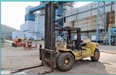
ale Model GDP250E Diesel Pneumatic Tire Lift Truck
