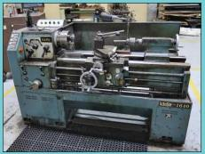
16" X 40" Victor Model 1640 Geared Head Toolroom Engine Lathe
