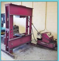
100 ton(est.) Enerpac Electric Hydraulic H-Frame
