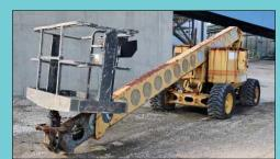
Grove Model AMZ66 Gasoline / Propane Powered Four-Wheel Drive Boom Manlift
