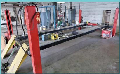
12,000 LB Ammco Model S412CXSORI Drive on Type Vehicle Lift
