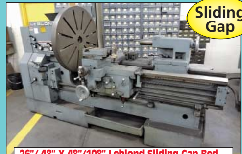
26" / 48" X 48" / 108" Leblond Sliding Gap Bed Lathe
