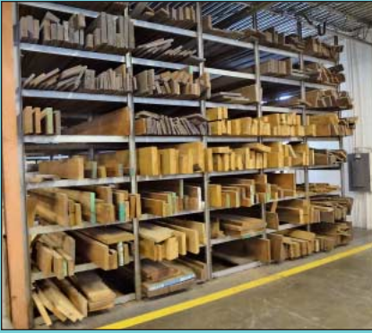
Large Quantity of Various Wood Used in Pattern Making; Mahogany, White Pine, Maple & Others
