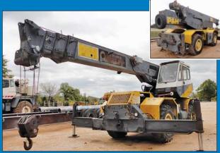
20 Ton P&H Omega 20 Model OM-20 Rubber Tire Hydraulic Diesel Rough Terrain Crane
