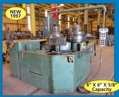
6" X 6" X 5/8" Roundo Model R6S R-6-S Horizontal Hydraulic Angle Bending Roll
