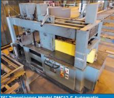
36" Trennjaeger Model PMC12-F Automatic Upacting Cold Saw
