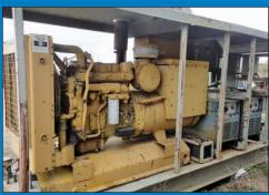
Caterpillar Model 3304 Diesel Power Gen Set w/ (4) Miller Arc Welders
