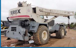
Backside of 50 Ton Terex RT-450 Rough Terrain Crane
