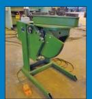
2,000 Lb. CWI Model P200F Tilting and Rotating Welding Positioner
