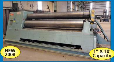
1" X 10' Roundo Model PS-360 Double Pinch Hydraulic Plate Bending Roll
