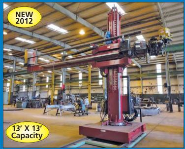
13' X 13' Key Plant / Red-D-Arc Model THD-5MX5M Welding Manipulator
