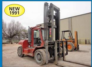
25,000 Lb. Taylor Model TE-250S Pneumatic Tire Diesel Forklift
