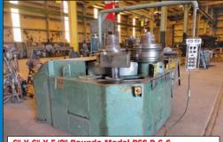
6" X 6" X 5/8" Roundo Model R6S R-6-S Horizontal Hydraulic Angle Bending Roll
