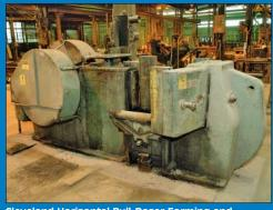
Cleveland Horizontal Bull-Dozer Forming and Straightening Press
