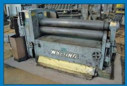
60" Wysong Initial Pinch Mechanical Power Plate Bending Roll
