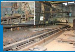
ESAB Model 200D Oxy Acetylene Three-Torch Plate Burning Table
