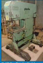
(2) 120 Ton Piranha Model SEP120 Single End Hydraulic Plate Punches
