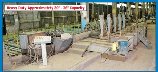
Hirschfeld Heavy Duty Five-Cylinder I-Beam Cambering Machine
