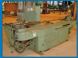
3/4" Pines Model M-725559 Horizontal Hydraulic Tube Bender
