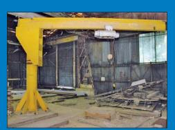
2 Ton X 16' Arm Floor Type Rotating Jib Crane
