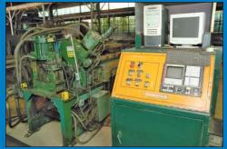
Peddinghaus Model APS-C21D Hydraulic Angle Shear and Punch Line
