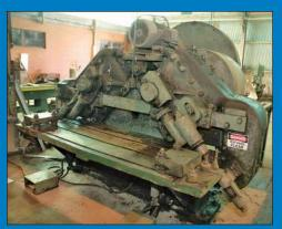
King Mechanical Bar and Angle Shear
