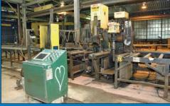
Controlled Automation Fabriline Model 3456-179 Automatic I-Beam Punch Line
