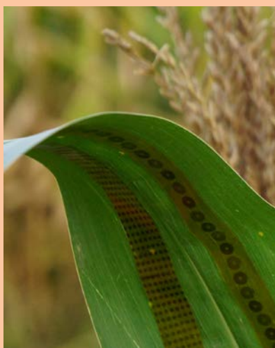
New sensors applied directly to the plant take real-time measurements of crop water usage. Image source: Liang Dong (Iowa State University).
