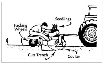
There are many types of tree-planting machines, but generally they have a coulter that breaks through the soil surface, a V-shaped blade that opens a trench into which the trees are placed, and packing wheels that firm the soil around the tree.
