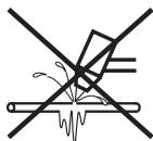
**A PLASMA ARC CAN DAMAGE FROZEN PIPES**
