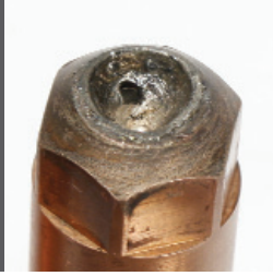
Fully-used OEM electrode after 1,100 starts
