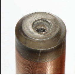
Partially-used SilverLine electrode after 1,500 starts
