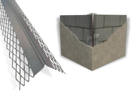
Angle beads provide with its solid metal nose a straight corner. Expanded diamond mesh wings allow for keying the plaster right up to the nose of the bead. It is designed to protect the corners.
