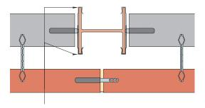
Stainless steel wall tie manufactured in accordance with BS EN 845-1
