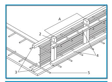
Fig 1 Straight expansion joint with Hy-Rib
