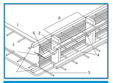
Fig 3 Expansion joint with Hy-Rib and joint band
