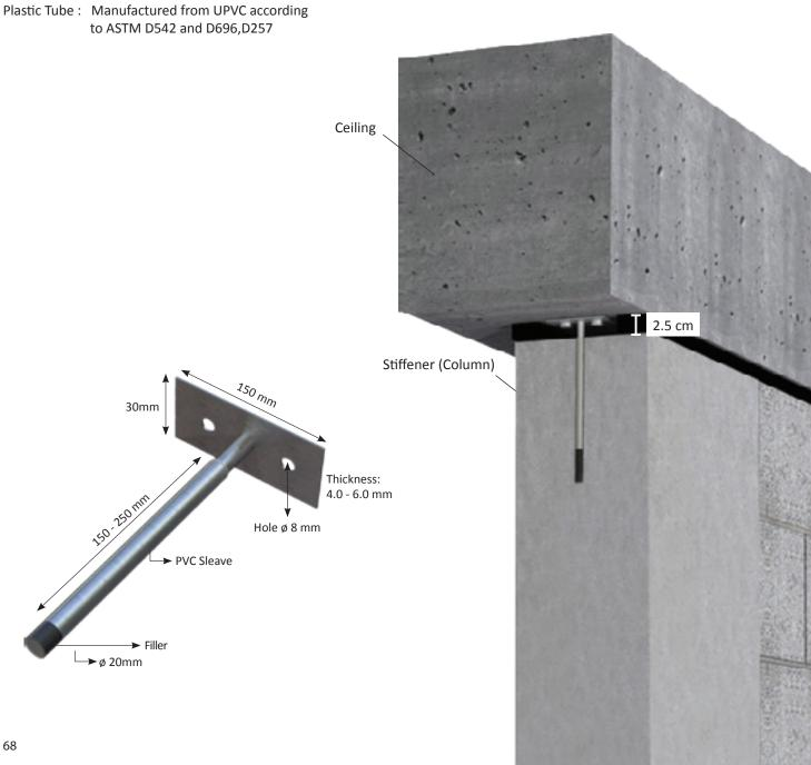
Partition Top Anchors have been developed to provide lateral shear resistance at the upper limit of masonry walls.
