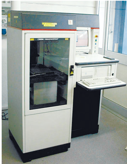
Figure 5.10 An SLA rapid prototyping system. (Courtesy 3D Systems, Rock Hill, SC)
