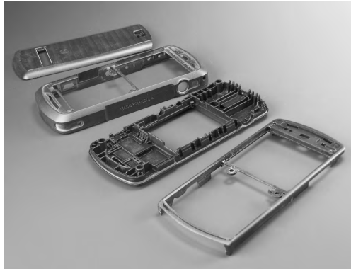
Figure 5.5 Prototype housings for a Motorola smart phone machined from molded blocks of 30 % glass-filled polycarbonate (Courtesy Motorola Rapid Prototyping Services)
