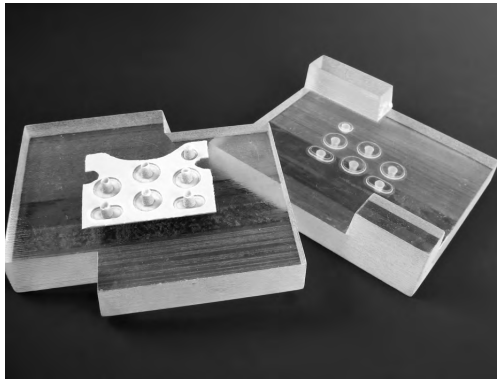
Figure 5.26 Prototype keypad for a Motorola Talkabout Radio cast from 40 Shore A durometer RTV silicone using a casting mold printed on an Objet EDEN 500 polyjet printer (Courtesy Motorola Rapid Prototyping Services)
