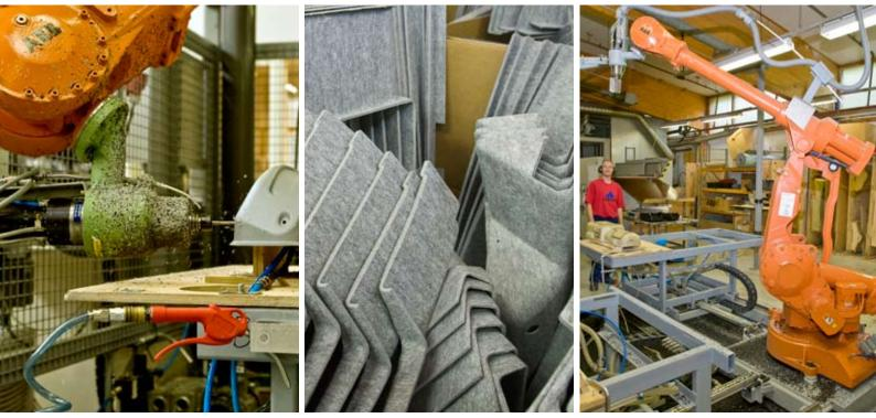
With robots, 150 parts per hour can be sawed versus 15 when done manually.
