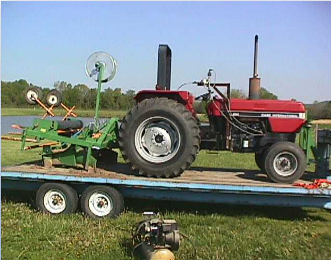
Kennco Superbedder and Reddick bedders throw up some of the highest beds.
