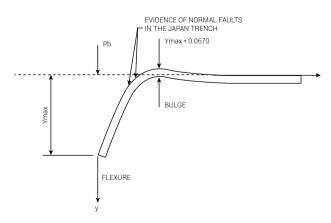
Figure 3. Flexure of a Semi-infinite Beam based on the equation  $Y = (Ymax) e^{-\lambda x} cos \lambda x$  (after Watts<sup>11</sup>).
