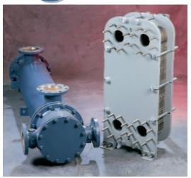
These attributes allow Plateflow to perform with one-third to one-fifth the surface area of a conventional shell and tube heat exchanger for the same application. The superior heat transfer capabilities make Plateflow an exceptional choice for heat transfer applications like heat recovery, applications with viscous fluids and large temperature cross situations.
