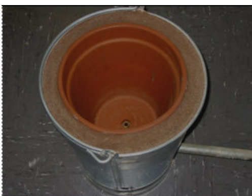
Finished Pellet roaster, minus wire-mesh basket.
