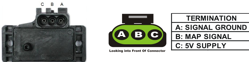
Figure 5 – Manifold Absolute Pressure Sensor and harness Termination
