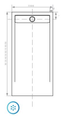
COTAS DESAGÜE A = +-120 mm /70/80 COTAS DESAGÜE A = +-140 mm /90 GROSOR B = 30 mm
