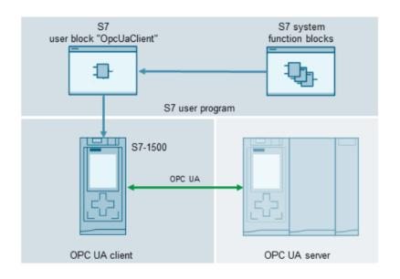
Open Standard useful for 3<sup>rd</sup> party card Client can use Registered Read/Write and Methods Setup is a combination of hardware and software blocks Data is available from Auto configured data blocks
