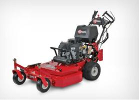
Gas Carbureted Standard Engine Manufacturer's air filter Yes Manual cutter housing and front caster spacer position adjustment. **Belt-Drive** Direct drive from transmission to double-belt wheel drives Kawasaki® 603cc FS481V V-Twin 3,600 rpm Carbureted 5-gallon (18.9-L) fuel tank. Lever-actuated blade engagement with blade brake. 2.0 mph (3.2 kmph) to 6.2 mph (10 kmph) forward, reverse assist.
