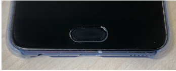
Figure 3: Home button covered with lip balm to prevent the fingerprint sensor from recognizing the users' fingerprint.
