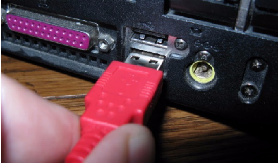
FIGURE H.4 Pictorial view of connecting the PICkit™ 3 to the USB port
