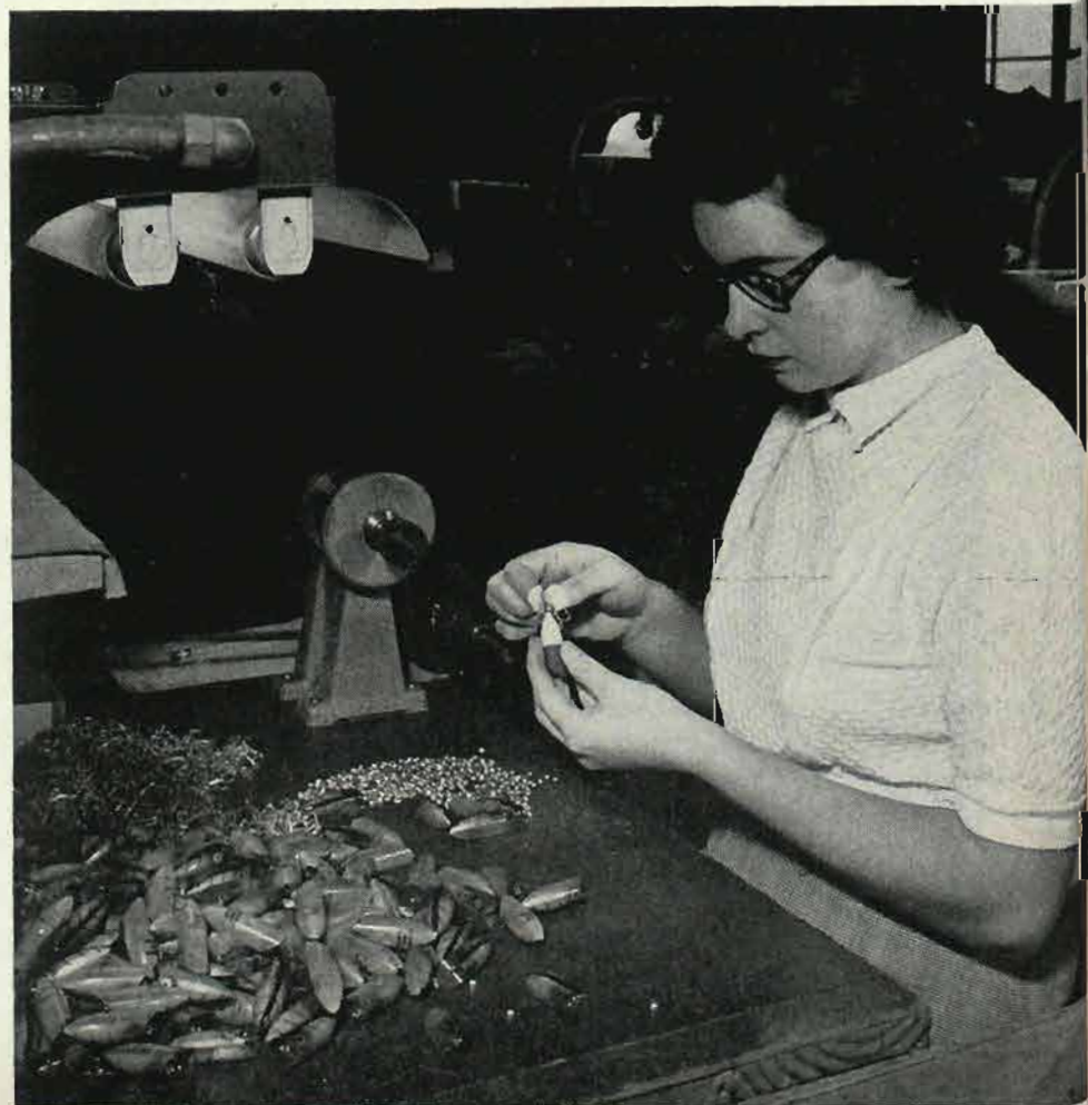
HOOKS ARE SHARP and this young lady wears the badge of her trade, a strip of adhesive tape protecting the fingers as she sets the hooks in place. Good lighting is highly necessary in the bait-making industry, promotes good craftsmanship.
