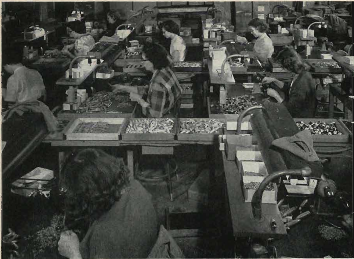
ASSEMBLY of the varied styles and patterns of lures for hooks, headpieces, guards and glass eyes is shown in this department where a woman's deft fingers make a speedy job of the most delicate operations. Note the electrically powered drills and screw driver machines on bench at lower corner.
