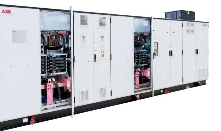
On the vessel side, each inverter unit (INU) is connected to a separate winding of the output transformer, with the load-side windings in series connection to form the desired load-side grid. This series connection, combined with phase shift-
