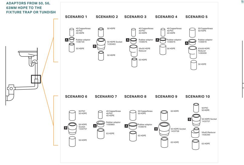
A: Can generally be fitted after the main pipe work has been installed, but before the floor coverings. B: Must be installed at the same time as the main pipework
