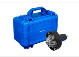
**GEBERIT PIPE SCRAPER D110** • For removing the oxide layer on Geberit HDPE pipes and fittings of size Ø110mm · For use with cordless screwdrivers Case to store pipe scraper
