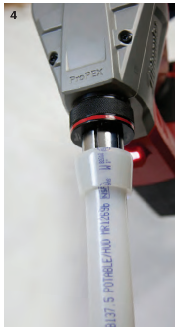
Expansion with Milwaukee M18 ProPEX Expansion Tool
