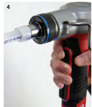
Expansion with Milwaukee M12 ProPEX Expansion Tool
