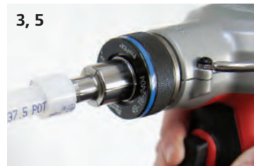
Expansion with Milwaukee M12 ProPEX Expansion Tool
