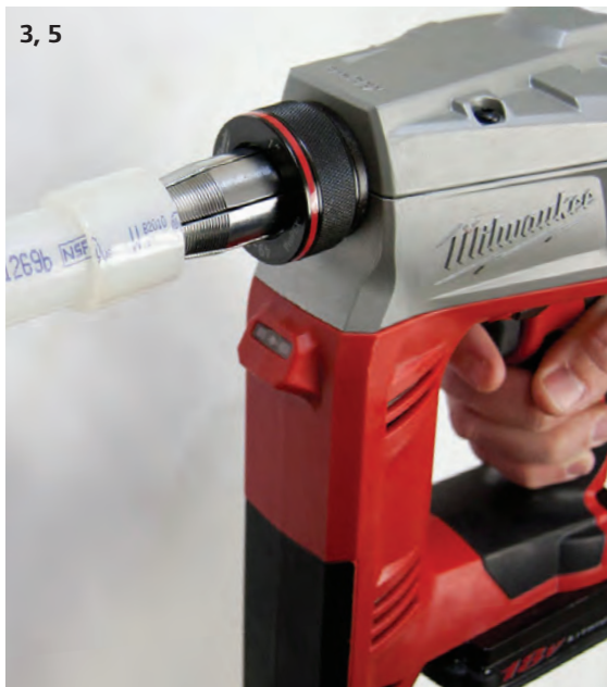
Expansion with Milwaukee M18 ProPEX Expansion Tool
