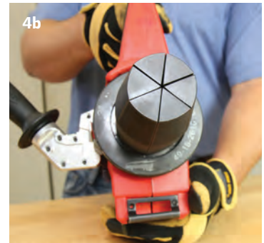
Correct Expansion Head Alignment
