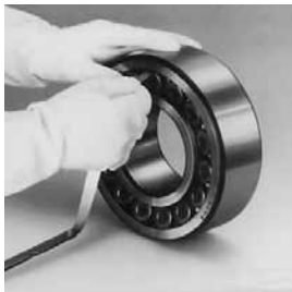
Fig. 1: Checking bearing clearance with bearing on bench.
