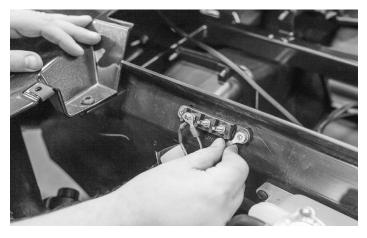
Connect the ring terminals to the factory accessory power distribution block. The power ring terminal gets connected to the ACC and the ground ring terminal gets mounted to the screw to the left.
