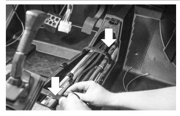
Continue routing the wire harness on top of the center console supports. Insert the plastic wire ties into the holes on the support bracing to secure in place.
