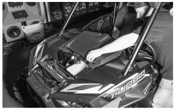
Using your hands, pull the top dash piece toward the interior of the vehicle to release it from the dash.
