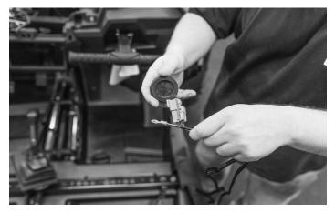
**Step 5 -Routing Wire Harness**Now that the center console is out of the way, take the wire harness and place it through the fire wall.
