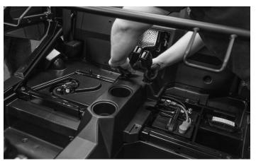
Next, remove the rear console if equipped (4 seater).
