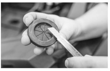
Remove the existing rubber grommet in the fire wall and cut along the score lines to open it up for the wire harness.
