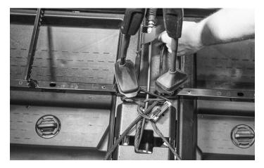
This kit is designed to work with Rockford Fosgate's RFRZ-RSW16 rear speaker wire kit. If you are using the kit, you will route the under the rear access panel. If you are not using the kit, simply wire tie the harness out of the way of moving parts or heat.
