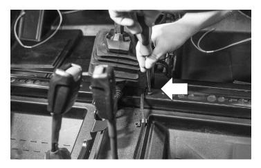
Remove the factory bolt and replace with supplied plastic clip.
