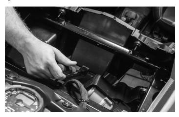
Be sure to slide the pocket support onto the rear brace for a secure fit.
