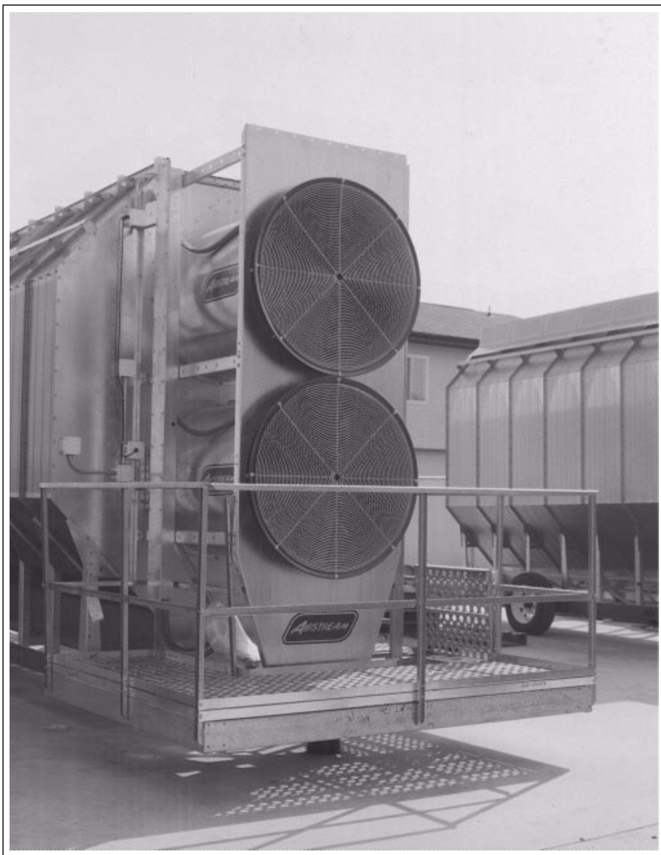
Figure 2AE Finished Platform on an Airstream Upper Module
