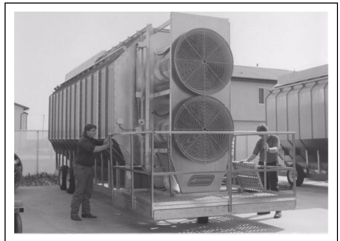
Figure 2AD Check to make sure every bolt is tight and door opens freely.
