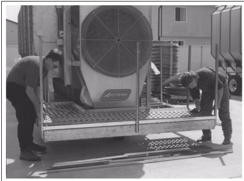
Figure 2U Installing Front Long Floor Panel
