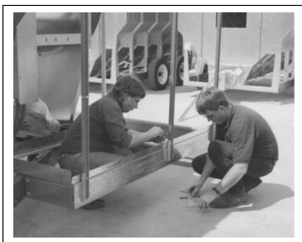
Figure 2Q Connecting Outer Front Toe Board to Guard Rail Support Channels
