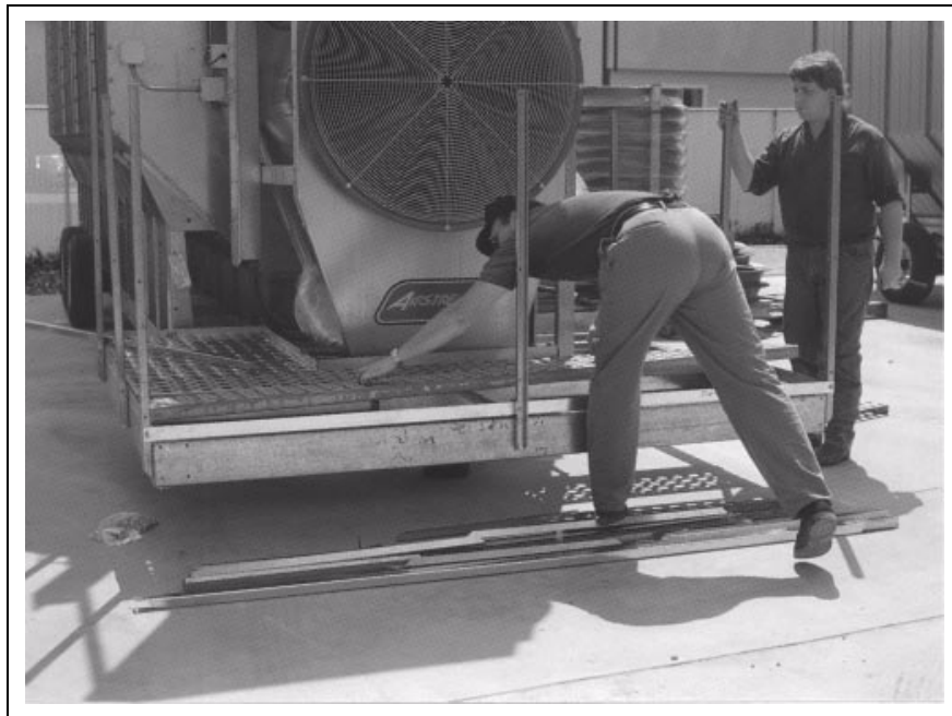
Figure 2T Installing Center Long Floor Panels
