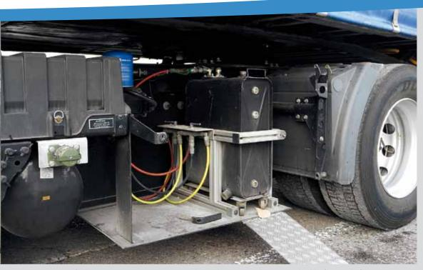
2 Precise fuel consumption measurement: the 30-litre test tank was weighed before and after each lap, then refilled.
