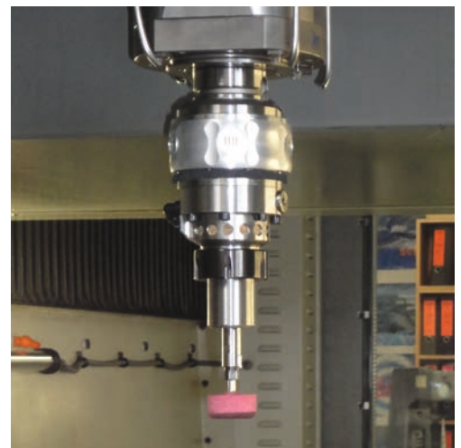
Example: RSC system in a machining centre
