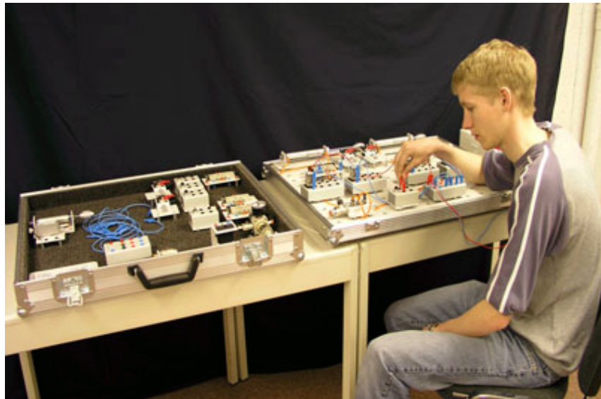
Typical portable with storage case trainer shown with Electro-Pneumatic components.
