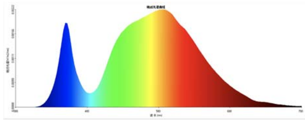
Figure 4 – Measured absolute spectral curve of subjects' eyes in scene A Figure 5 – Measured absolute spectral curve of subjects' eyes in scene B
