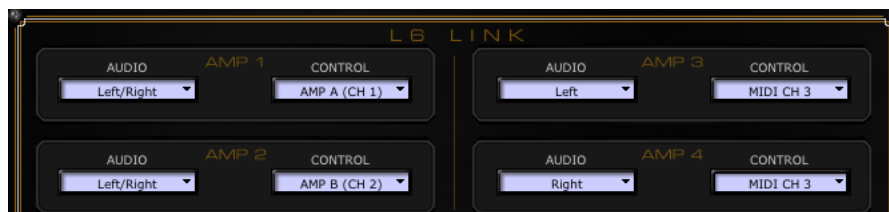
The L6 LINK Audio & Control options for up to four DT50 amplifiers
