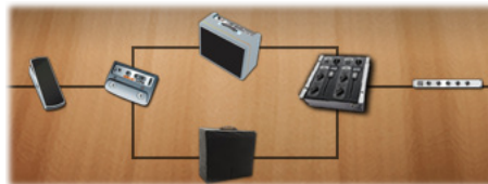
Dual Amps within Paths A & B - Amp B is in the "Null" (disabled) state
