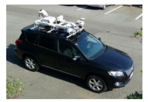
Figure 1. Mobile mapping system
