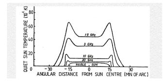
Figure 4. Sun Temperature at Microwave Frequencies
