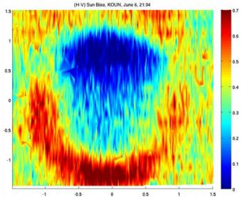
Figure 6. Differential Power Across the Solar Disk
