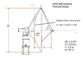
Figure 2. The WSR-88D Antenna Specifications
