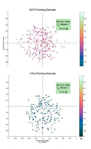
Figure 8. Sunspike Monitoring for Two Radars
