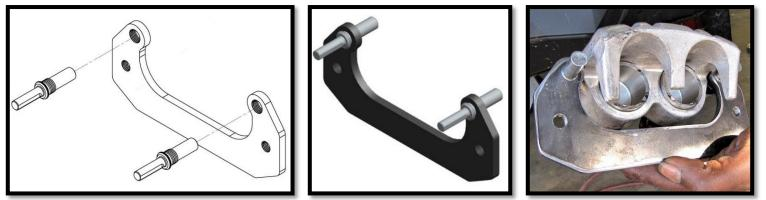
d. Install the caliper onto the portal box between the new caliper bracket and rotor. Use the factory mounting bolts. Position brake line banjo fitting so it runs at the proper angle for maximum suspension travel. Tighten & torque to specifications. (15mm) [30 ft lbs]
