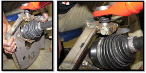
c. Properly position the lower ball joint into the lower ball joint mounting bracket on the backing plate assembly. Then fasten the front lower ball joint with the factory hardware. (15mm)[50 ft lbs]
