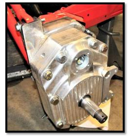
d. Loosely fasten the all bolts with **1/2**" flat washers and **1/2**" lock nuts. Recheck all parts that were used and make sure everything fits correctly, and then go ahead and tighten and torque all bolts. (3/4)[105 ft lbs]
