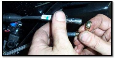
d. Install the new **61**" **FRONT LEFT** brake line to the banjo bolt. Run the line back through the frame and to the (DR) side hub.
