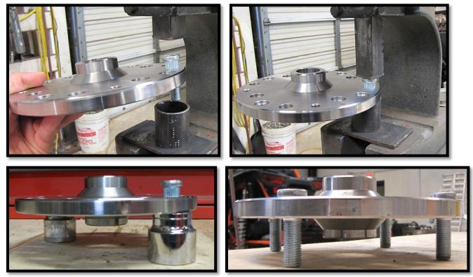
e. Once the studs are pressed in, place (4) <sup>1</sup>/<sub>2</sub>" brake rotor spacers PGLC-ROTOR-SP over the tapped holes.
