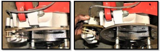
c. Disconnect the radius bars from the knuckle. (15mm)
