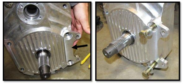
d. Slide a 1/2" flat washer onto (4) 1/2 x 4-1/2" bolts and insert them into the remaining four holes of the box.
