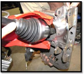
b. Install the backing plate to the trailing arm using M10-1.25x40 bolts, 10mm lock washers, and 10mm flat washers. Then fasten bolts with M10-1.25 lock nuts. (15mm) [56 ft lbs]
