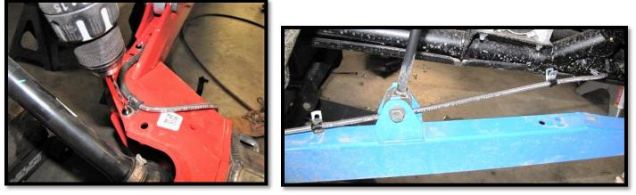
b. Disconnect BOTH rear factory brake lines from the rear brake line block. Have a container to collect fluid.
