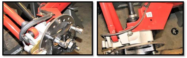
Remove the caliper mounting bolts from the rear hub and remove the caliper. (15mm)
