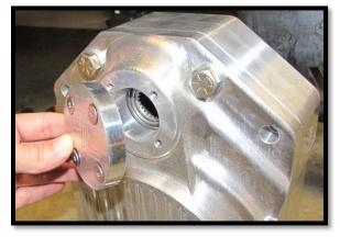
c. Find the caliper mounting bracket **PGLC-BCB-95K** and place it in the corresponding fitted <u>front</u> section of the portal box. Then insert a **1/2 x 4-3/4**" **bolt** and **1/2**" **washer** into the bracket holes & box.
