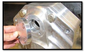
c. Find caliper mounting bracket **PGLC-BCB-115N** and place it in the corresponding fitted <u>FRONT</u> section of the portal box. Then insert a **1/2 x 4-3/4" bolt** and **1/2" washer** into the bracket holes & box.
