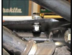
g. Secure the rest of the brake lines using **provided hardware below**. They should be routed down the same passage where the factory lines were. Make sure there is no binding in the lines once they are secured.
