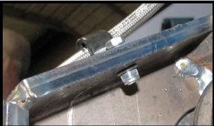
h. Use the supplied **zip ties** to reposition and secure the brake lines, then fasten the brake line back to the caliper. **Make sure there's no binding in the lines, even at full turn.**
