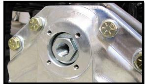
c. Align the portal box lid cap & gasket. Use the 1/4-20 x 3/4" screws and install to the box. (3/16)[8 ft lbs]
