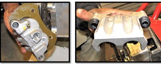
c. Find the new rear brake caliper hanger bracket **PGLC-BCB-85X.** Apply **LOCTITE (BLUE)** to the pins and fasten them to the bracket. [73 ft lbs] Then insert it into the brake caliper.
