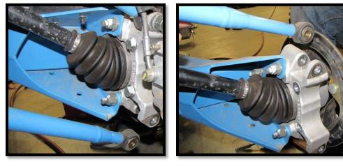
d. Remove the cotter pin and loosen the rear wheel hub castle nut (27mm). Remove the nut from the rear wheel hub assembly. Then remove the brake rotor assembly.
