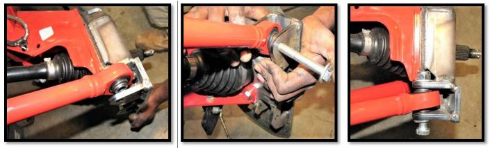
c. Slide a **12mm washer** onto a **12mm x 75 bolt**. Use it to reattach the lower radius bar. Secure it using a **12mm washer** and **12mm lock nut**. (18mm)[90 ft lbs]
