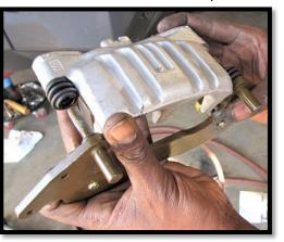
c. Find the new rear brake caliper hanger bracket **PGLC-BCB-108M.** Apply **LOCTITE (BLUE)** to the pins and fasten them to the bracket. [73 ft lbs] Then insert it into the brake caliper.
