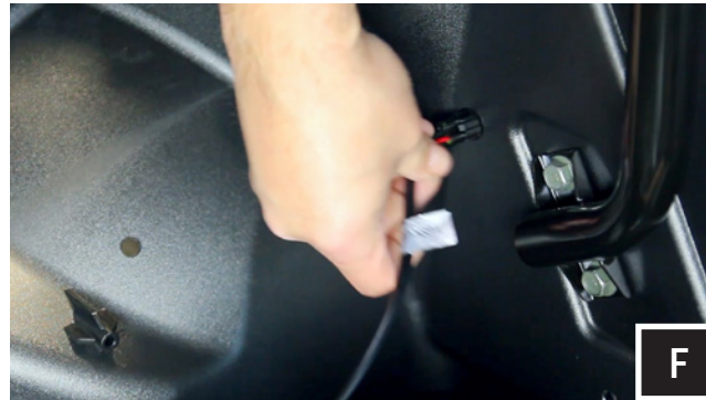
F. Route the speaker cable attached to the pod through the inside footwell 1/2" hole. Position the speaker pod in place and line up with drilled mounting holes
