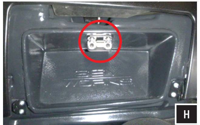
H. For 2014 model year vehicles remove the factory glove box door latch. Mount the latch to the supplied bracket and secure to the enclosure using the short screws provided
