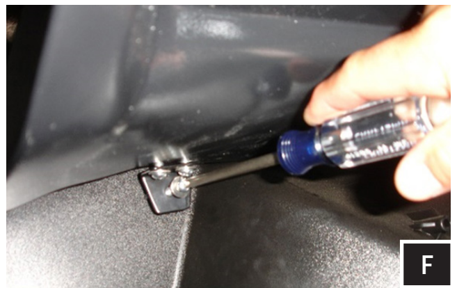
F. Loosely install the bottom L bracket, align the mounting hole with the factory bung and secure with one of the long screws provided (you will tighten the bracket to the enclosure and factory bung AFTER step H)
