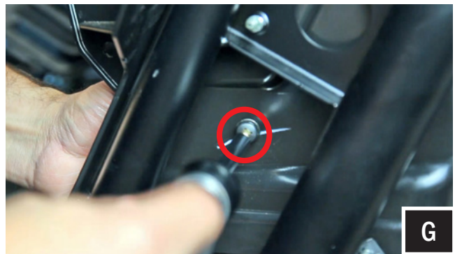
G. With the provided M6 screws and washers, loosely mount the pod through the 3 holes previously drilled. Once all screws have been inserted into the pod, hand tighten all 3 screws.
