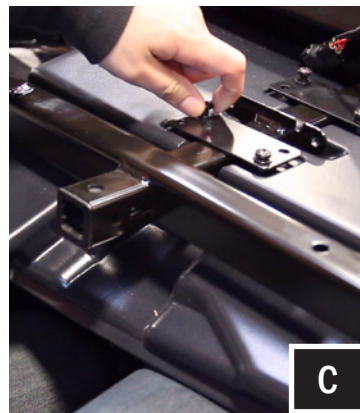
C. Lift the enclosure into place and align the top channel in the grab handle bar, while holding the enclosure in place, loosely attach the flat brackets to the top of the enclosure using the long screws provided.
