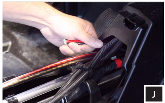
J. Feed the power wire through the grommet hole and back through the center console to the battery.
