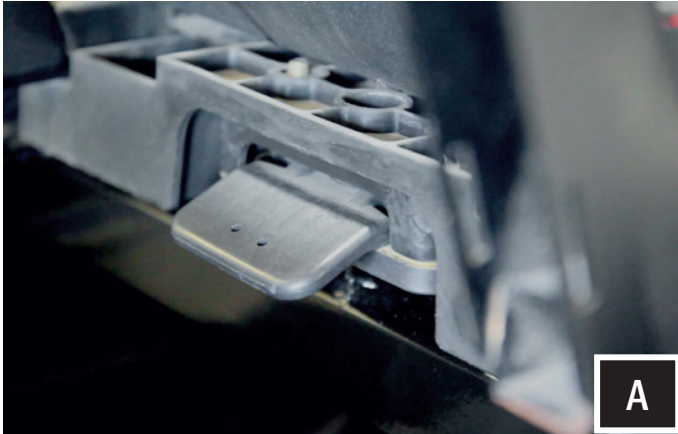
A. Remove all seats by releasing the handle behind each seat, push forward slightly while lifting up.
