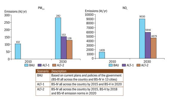
Figure 5: PM and NOx emission reduction in 2030 in vehicular sector due to introduction of BS-VI norms in 2020. Source: Sharma et al. (2014)
