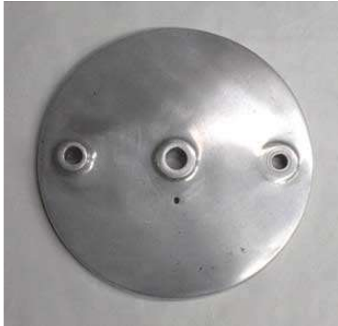
Figure 26. After 1 st Polishing Operation (cutting down) with Emery Cake
