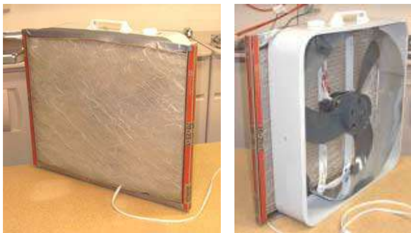
Figure 32. El-Cheapo Box Fan Dust Collector
